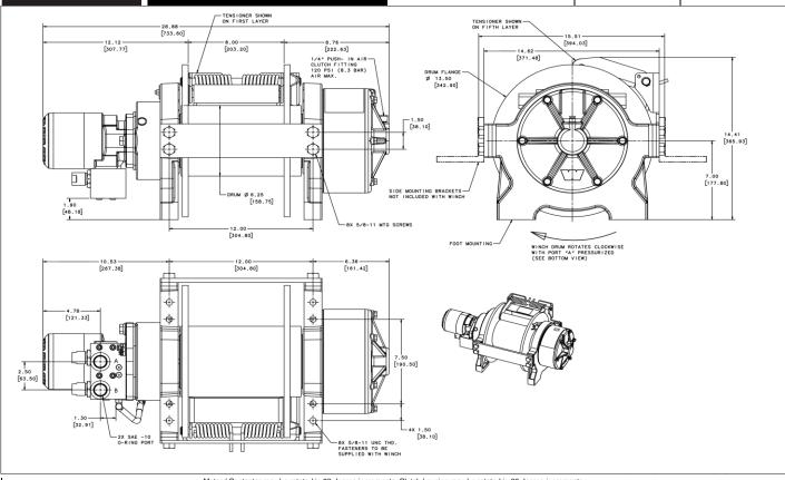
Motor / Contactor may be rotated in 90 degree increments. Clutch housing may be rotated in 60 degree increments.
